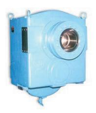
Elecon has already developed two defferent sizes of such gear boxes, viz 250 KW and 55 KW respectively for M/s NEPC Micon & BHEL Hyderabad. These gear boxes are coaxial and (Wind Turbine) shaft mounted working at 40 Mtr high on the tower. The internals are carburised, hardened and ground and specially profile corrected for speed increasing gear application. The toothing and bearing are bath/ splash lubricated and gear boxes fixed on the turbine shaft by means of shrink disc.
